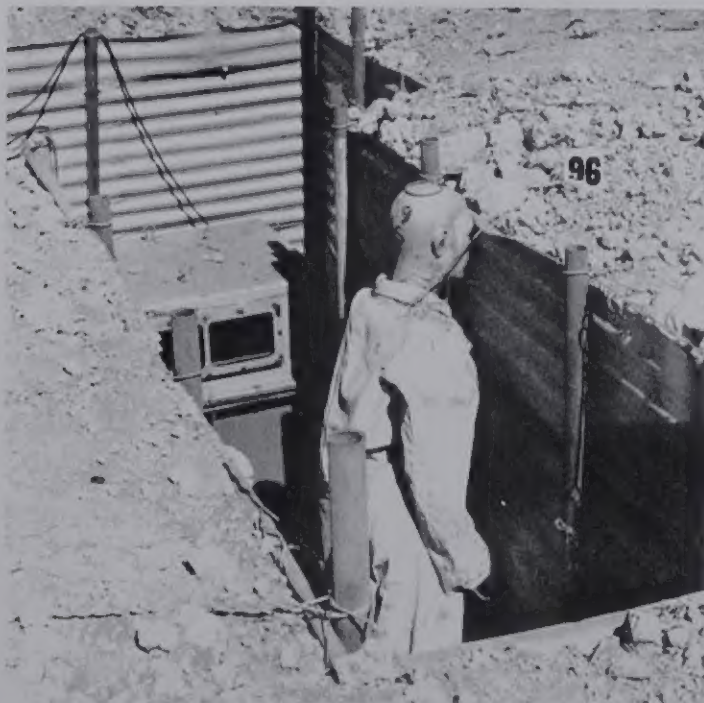
FIGURE 24. DUMMY IN TRENCH AT 2390 ft AFTER FIRING
